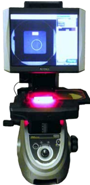
The resin flows into the circle during lamination and the final diameter of the circle is measured (see Figure 2 and 3). The difference between the original 1.000” diameter of the circle and the final diameter is the amount of flow in mils. By this method (IPC TM650 2.3.17.2), a typical Low-Flow material may have anywhere between 0.030” and 0.120” of flow, depending on the grade and the degree to which the flow is restricted in the resin formula and treating (prepregging) operation.
